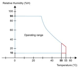
Red: Extended temperature range of 7-15" devices; see section "Selecting a mounting position (Page 14)".
