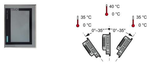
A maximum ambient temperature of +40 °C is permitted for vertical mounting (0° tilt angle); a maximum of +35 °C is permitted for inclined mounting.
