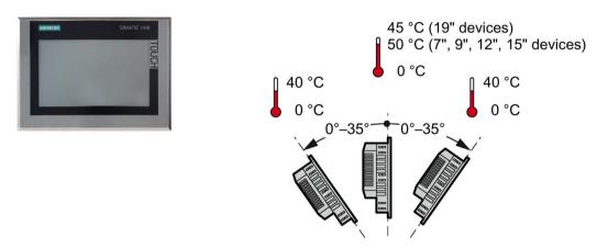
A maximum ambient temperature of +50 °C is permitted for vertical mounting (0° tilt angle); a maximum of +40 °C is permitted for inclined mounting.
