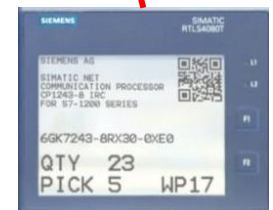
RTLS Transponder with e-paper and 2-way communication
